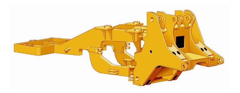
**Engine End Frame.** Is a full box section frame with hitch plates at the front end that provides a strong, rigid structure which resists twisting and impact loads. Rear counterweight mounting, battery box and toolbox are located at the back of the frame area.
