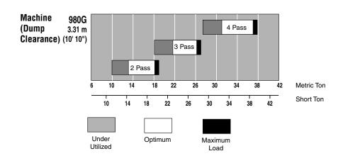
Truck Match. The 980G Series II is an aggressive first gear loader for face and bank excavation, but the versatility of a material handler was also designed into it. With increased rimpull and full match torque converter in second gear, the 980G Series II is an aggressive second gear stockpile loader. With ample dump clearance, it can easily load on-highway trucks in two to three passes and offhighway 36 tonnes (40 ton) trucks in four passes.
