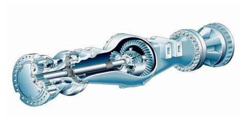
**Axles.** Are fixed on the front and oscillating ±13 degrees on the rear. The design meets the demands of Ride Control and autoshift that often result in higher speed load and carry applications.
