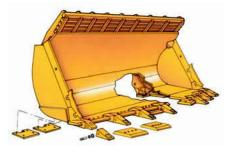
Bucket Construction. Caterpillar General Purpose and Rock buckets feature proven shell-tine construction for maximum performance and durability. Tines reinforce the bucket floor from the hinge plates to the cutting edge, forming box sections that provide protection against impact and twisting forces. Integral spill plates provide better material retention and maintain operator visibility. Rackback stops protect the buckets from damage and impact forces.
