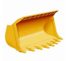
Rock Buckets. Are designed for use in face or bank loading and feature a high penetration spade edge for greater impact loads and/or increased material penetration. Added wear strips reduce the need for costly bucket rebuilds. Select from BOCE; penetration teeth; shouldered, double-strap sidebar protectors; and mechanically attached wear plates (MAWP) in place of standard wear plates to meet the needs of specific applications.
