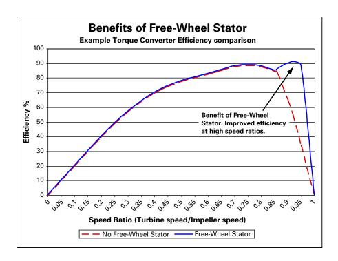
Free Wheel Stator Benefits. The graph represents the efficiency of a fixed torque converter relative to an equivalent converter with a free wheel stator. When the turbine/impeller speed ratio of the two converter types is below
