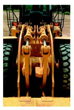
Linkage. Lift arms are solid steel, providing superior strength with an excellent front end viewing area. The proven design offers excellent dump clearance and reach for exceptional matching to both on- and off-highway trucks. Z-bar linkage generates excellent breakout forces and good rack back angle for better bucket loading and material retention.
