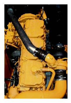
**Engine.** Is a six cylinder, turbocharged and aftercooled 3406E Electronic Unit Injector (EUI) which is powerful enough for the most demanding work.
