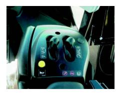
**Bucket Controls.** Electro-hydraulic (E/H) bucket and work tool controls offer precise lift, tilt and auxiliary control with extremely low operator effort. The armrest and console can be moved vertically or fore and aft. The hydraulic control console can also be tilted, and the wristrest can be adjusted vertically.
